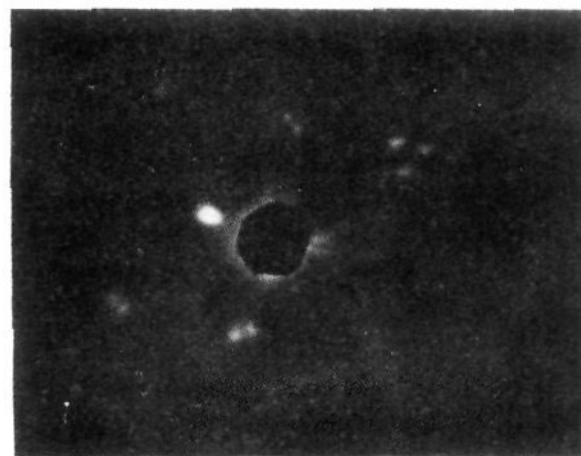
Figure 4. Photograph of the LEED pattern obtained by heating \text{CH}_3\text{NC} to \sim 375 K. The ring of split spots around the (0,0) beam are 1/4 order diffraction spots. The dark circle is from the glow of the electron gun.
